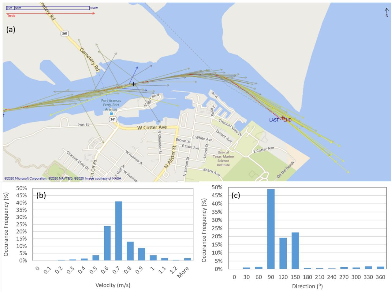
Figure 2-3. Depth-averaged current ( $U_{95}$ ) during slack to ebb tidal stage in the CCSC between Harbor Island and Port Aransas. (a) Spatial and (b-c) statistical distributions of speed and direction of  $U_{95}$ . The direction of  $U_{95}$  refers to the current heading measured clockwise from true north. Field current measurements were conducted on September 22, 2019, from 11 AM to 12 PM.
