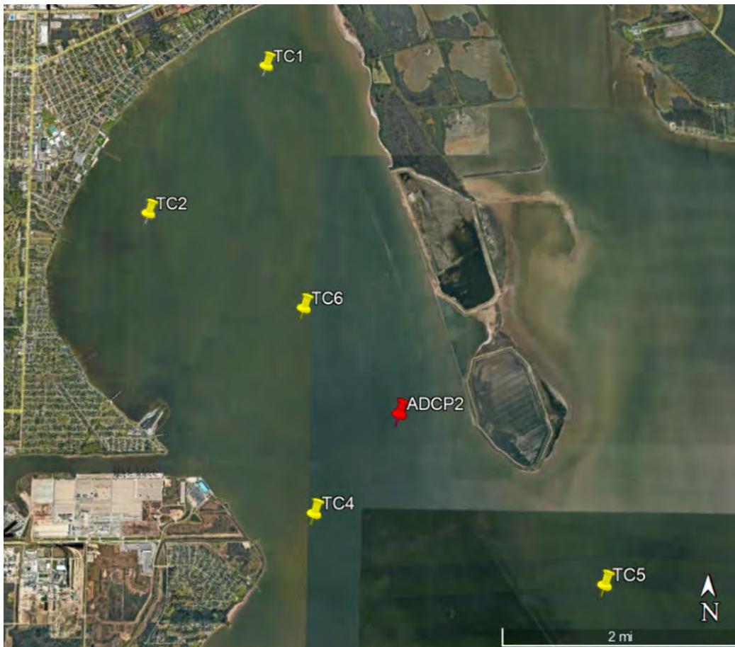
Figure 4-3: Locations of fixed instruments deployed 15-28 April 2022. Yellow pins indicate TCM and RBR pressure transducer pairs. The red pin indicates a bottom mounted ADCP.
