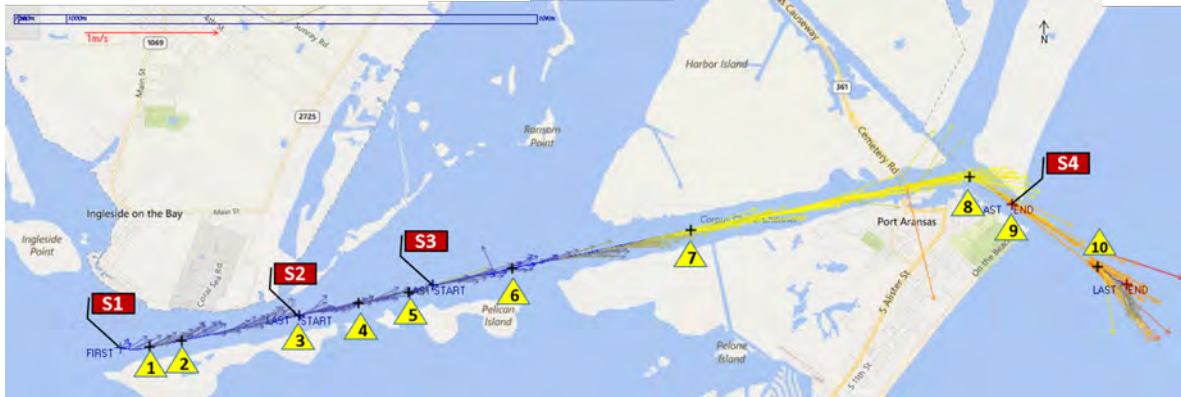
Figure 3.1: Depth-averaged current vectors U_{95} for segments S1 – S4 during east bound survey between Port Ingleside and Port Aransas.
