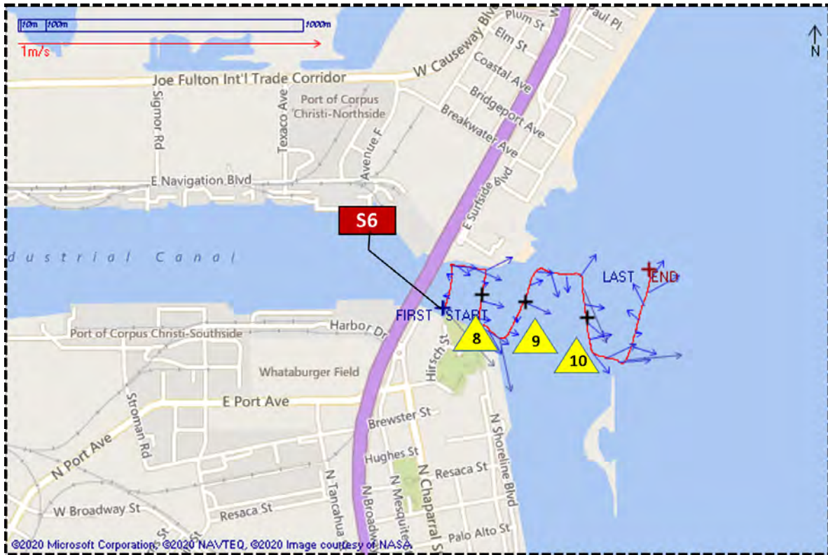
Figure 3.40: Depth-averaged current vectors U_{95} for segment S6 at the harbor entrance measured on 9/23/2019.
