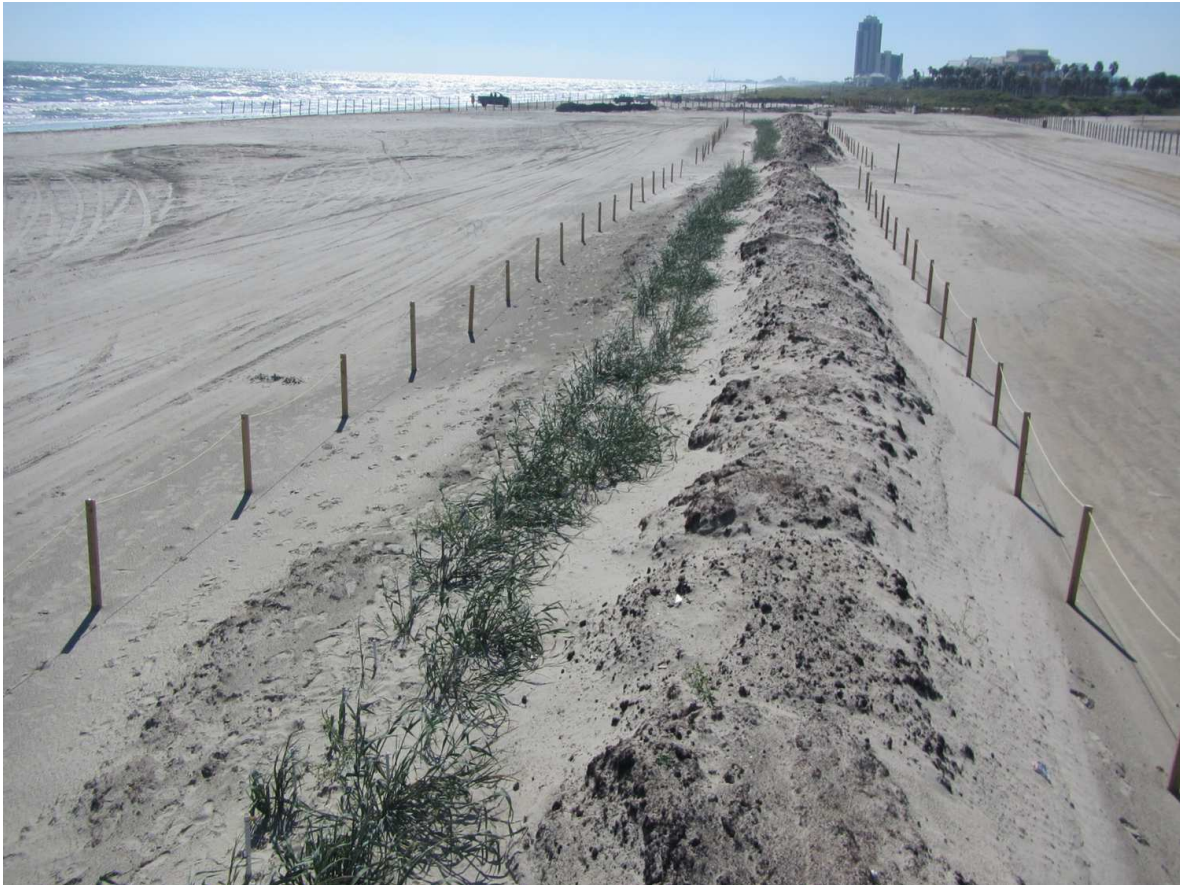
Figure 1.3: Photo of prototype dune nine weeks after vegetation planting. Each segment was roped off to avoid disturbance from foot traffic across the dune.
