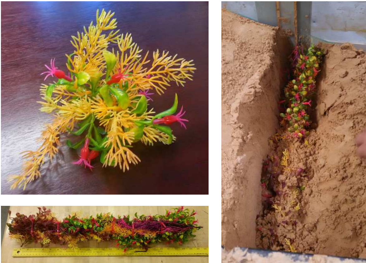
Figure 3.2: Photos of artificial seabed material used in flume testing. Off the shelf plastic aquarium plants were chosen to model the Sargassum seaweed. Individual pieces were glued together and buried inside the dune to simulate seabeds.
