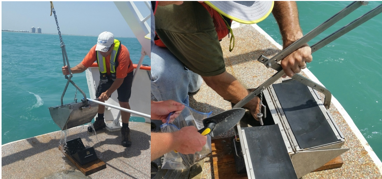
Figure 5. Photos showing the process of surface-sediment grab sampling at seabed locations. The grab sampling device was lowered to the seabed from the vessel. Collected sediment material was transferred to sealable plastic bags and catalogued.
