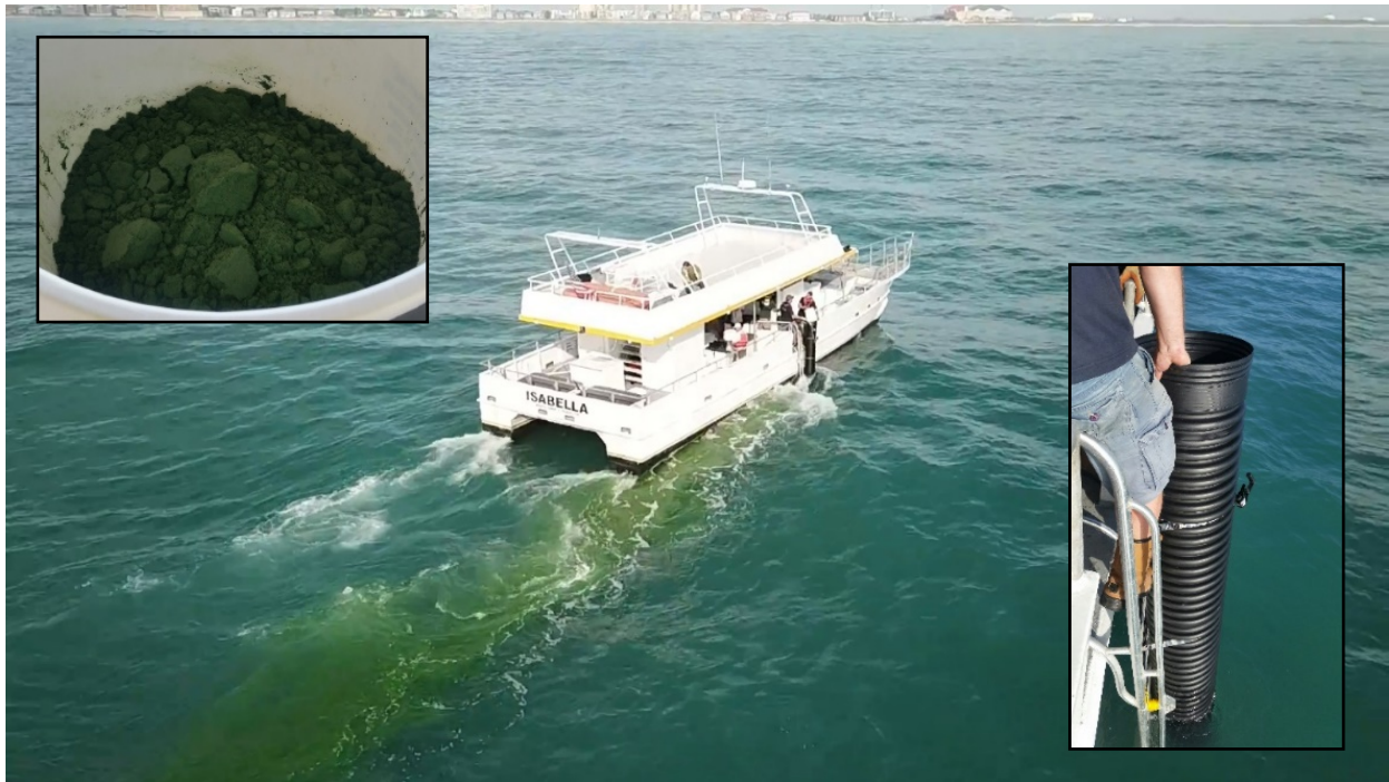
Figure 3. Photo of tracer deployment. 2000 kg (4,400 lb) of ferrimagnetic fluorescent tracer particles (top left inset) engineered to match the hydraulic characteristics of the dredged material were released via a chute on the side of the boat (bottom right inset) over the top of the nearshore berm in August 2018.
