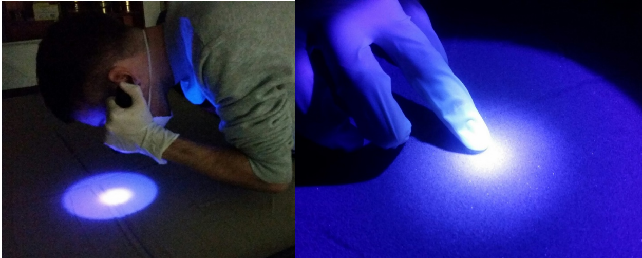
Figure 6. Photos of laboratory tracer count assessment using blue light illumination. Surface grab samples were dried and spread out on a flat PVC tray for that purpose.
