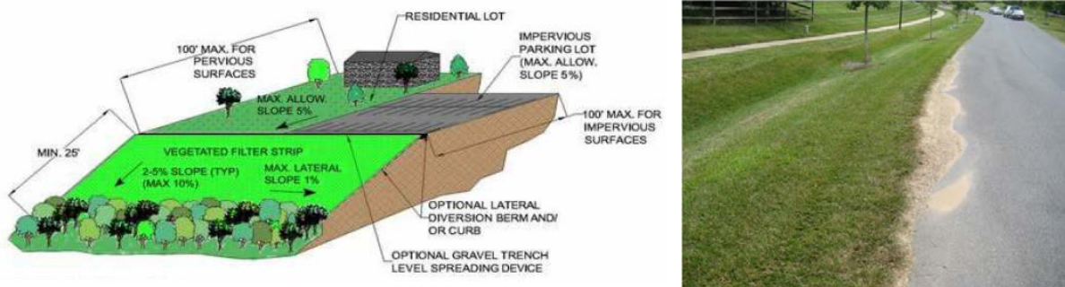
Figure 30. Schematic and photo of vegetated filter strips (VFS). A conceptual illustration of a VFS system (left, source: Pennsylvania Stormwater Best Management Practices Manual, 2006), and an urban VFS providing a buffer between an impervious roadway and a vegetated swale (right, source: Chesapeake Stormwater Network).
