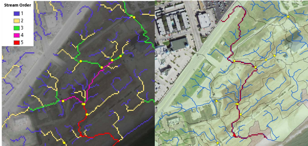
Figure 5. Example of stream ordering and a longest pathway throughout the stream network within the beachside runoff catchment for the east project area on Galveston Island. The low-order streams associated with overland flows converge to form higher-order streams on the beachside downstream area (left panel). Note that the transparency of the background DEM raster was adjusted for visual display of the underlying areal image. The longest flow path (dark-red, dotted-line) across the respective stream network (blue lines) is determined (right panel) to later estimate the time of concentration, t_c . Mid-pour points (●) are specified at the junctions between the high-order (third- or higher-order) stream links. The peak runoff rates are evaluated at the pour points (▲) located at the downstream end of the converged main streams of the respective runoff stream network.
