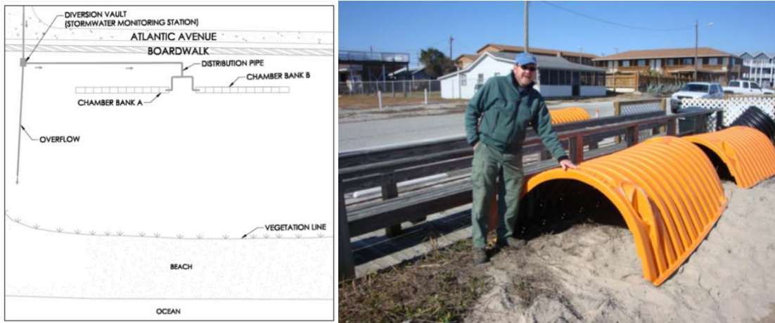
Figure 24. Layout and photo of a North Carolina dune infiltration systems. A general layout of the dune infiltration systems (left) and a photo of open-bottom chambers for underground storage (right, source: NC State Extension available at www.ces.ncsu.edu ).
