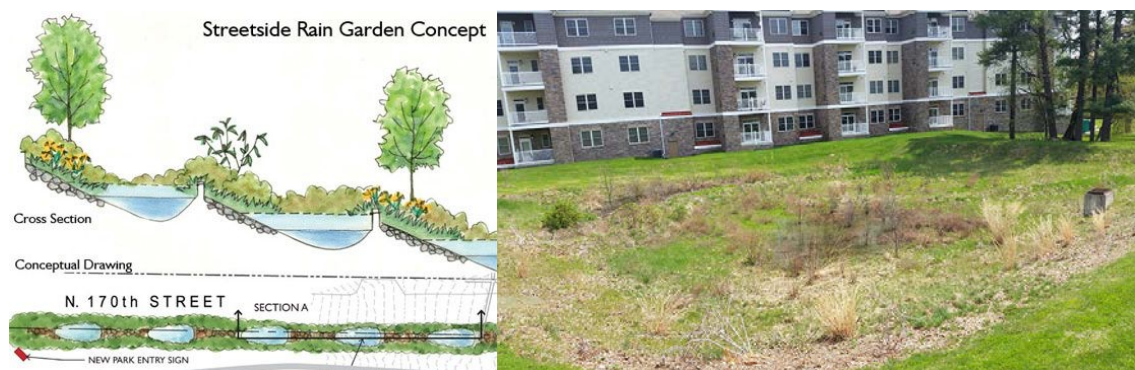
Figure 23. Schematic and photo of examples of berms and retentive grading in urban settings. A street side rain garden concept implementing diversion berms created by shallow depressions on the upslope (left image, source: Pinterest) and retentive grading in a residential area in Philadelphia (right image, source: Philadelphia Water, 2015).
