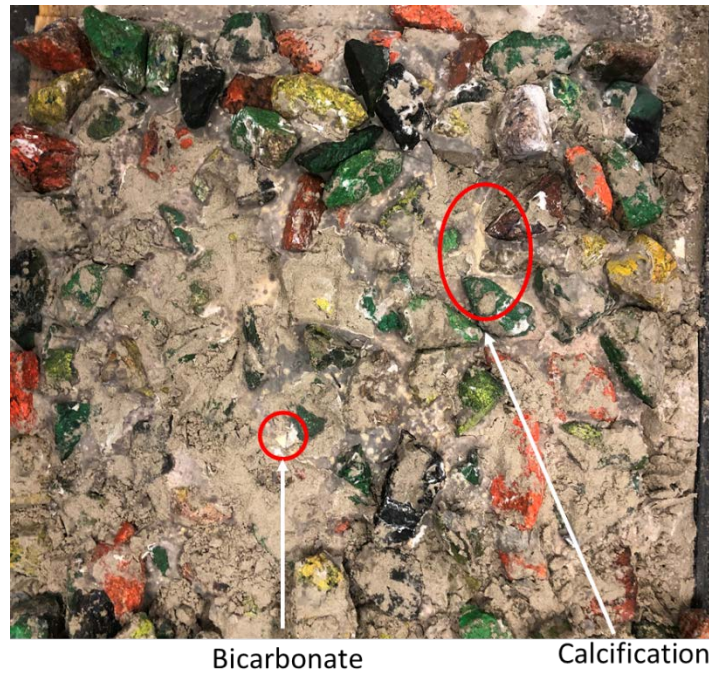
Figure 4-3: Visual evidence of calcification in MICP-treated rock-sand matrix after complete slope failure of test (iii). Calcification is visible as an off-white color while remaining pockets of sodium bicarbonate deposits are bright white.
