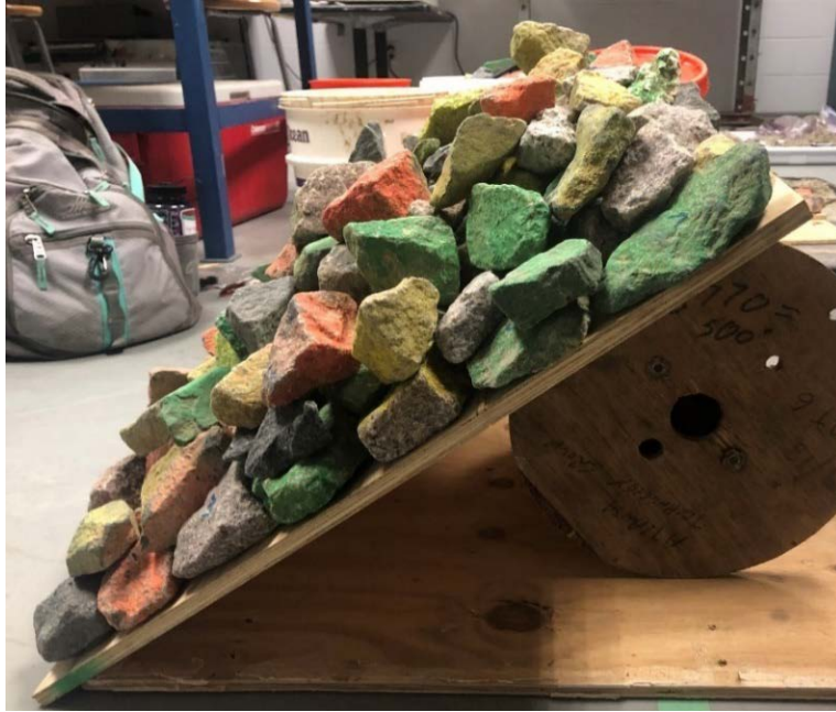
Figure 4-2: Slope Test Setup shown for the test involving rocks. The wire spool was used to increase the height (and therefore slope) of the rock matrix.
