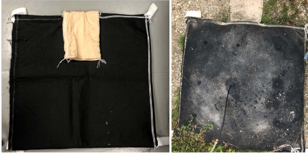
Figure 4-1: Photo of geo-synthetic bag made of Mirafi S3200 material. Left panel: empty bag prior to filling. Right panel: bag with evenly distributed button drippers inserted into the geofabric surface.
