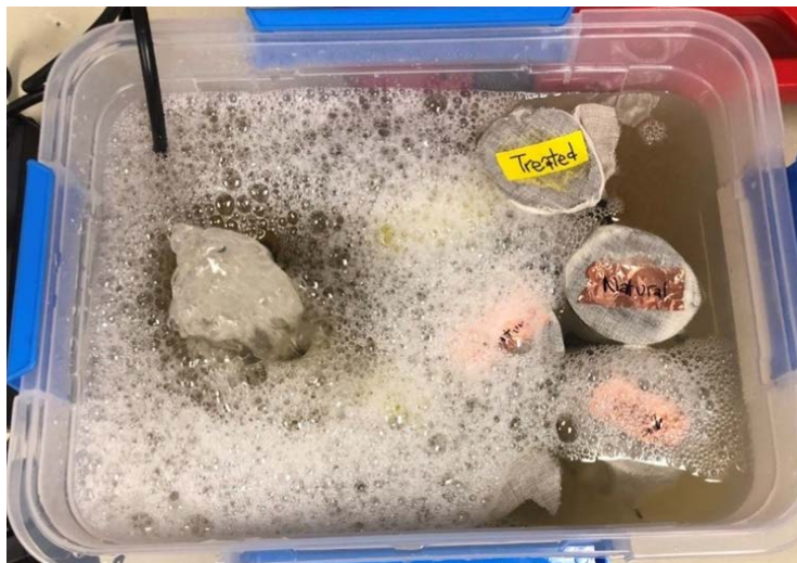
Figure 2-2: Experimental setup of cylindrical mesh molds submerged in MICP solution. Molds were created from wire mesh and were filled with autoclaved and natural sand from Dellanera Beach.
