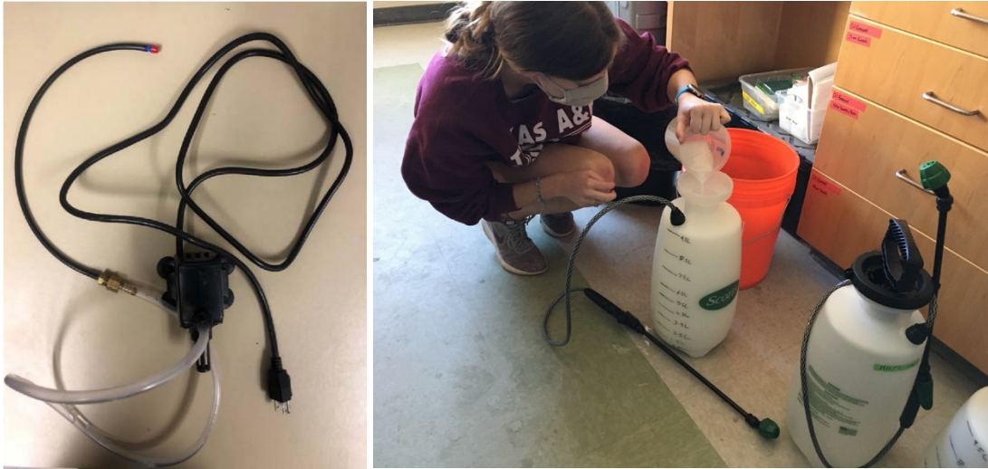
Figure 3-2: Photos of two different MICP solution delivery systems for field experiments. The left panel shows the pump, hose, and nozzle setup. The right panel displays the graduated manual sprayer containers being filled with MICP solution prior to a field test.
