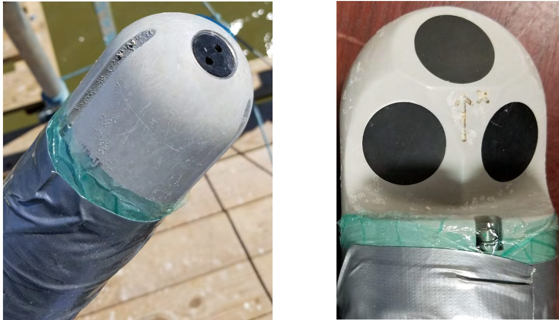
Figure 3.5: Photos of ADCP pressure transducer (black circle in left panel) and ADCP head with three velocity transducers (right panel).
